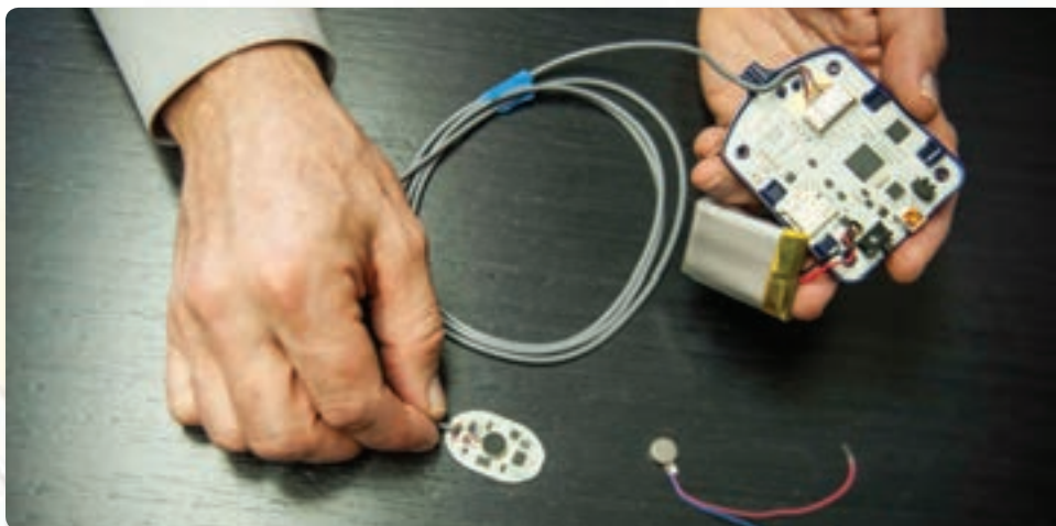
The inner workings of Sanger's electromyographic device, which monitors the electrical current generated by muscle movement
